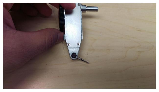
6. Zero the dial indicator by holding the outer rim and rotating the face
