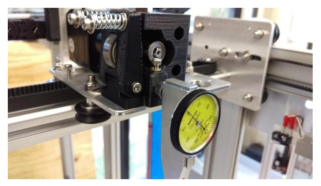
9. Keeping the dial indicator as vertical as possible, lock it into place by tightening the M3 SHCS set screw with the 2.5 mm Allen Key
