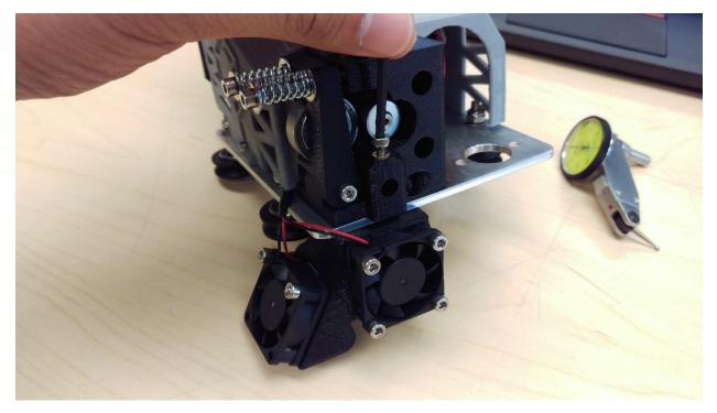
8. Insert the shaft of the dial indicator into the cavity at the front of the extruder assembly
