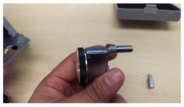
4. Hand tighten the shaft to lock it into place
