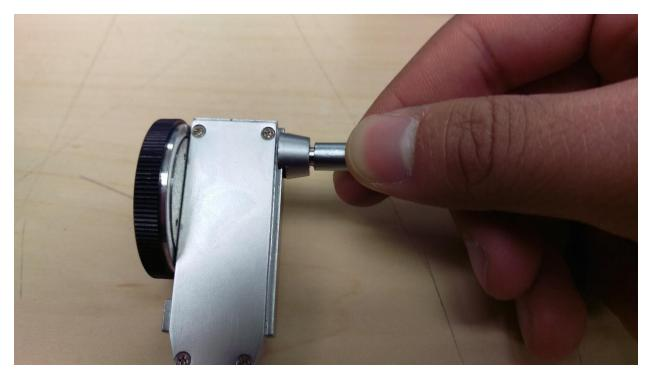
5. Swivel the arm of the dial indicator so it is about 20 degrees away from the horizontal as shown
