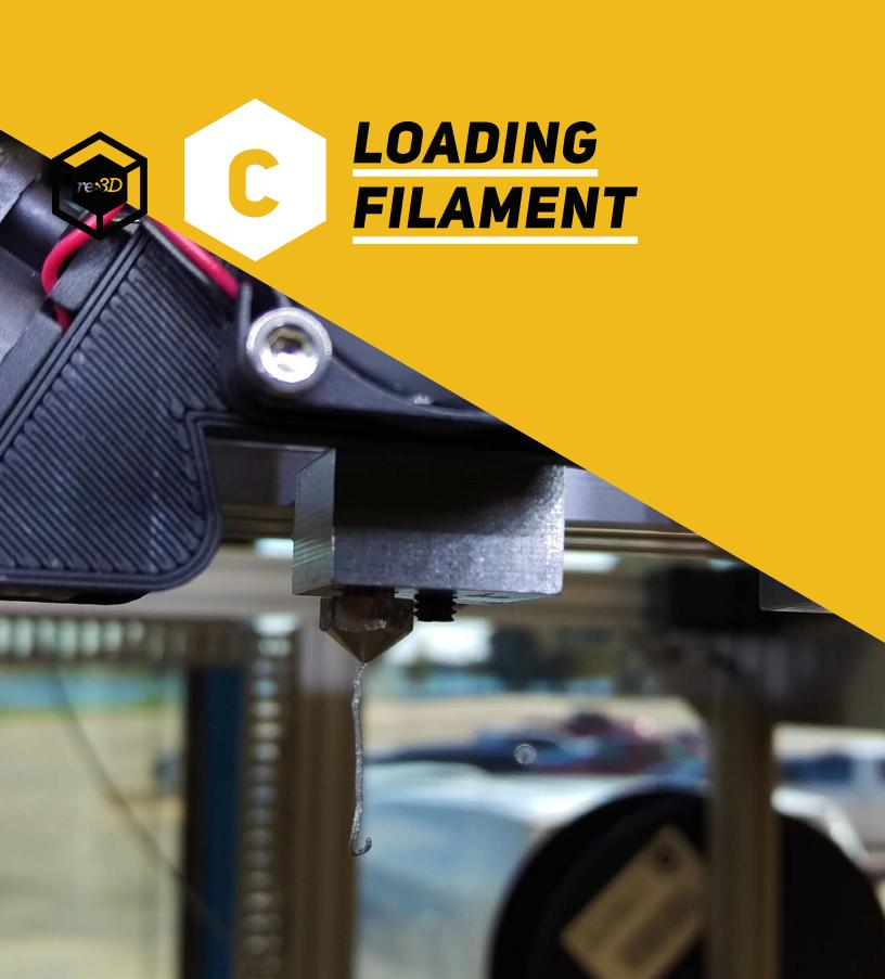
Gigabot® prints with 2.85mm diameter plastic filament. Thanks to the all-metal design of the hot ends, Gigabot users can print virtually any 3D printing filament available on the market! The following section demonstrates how to load filament to Gigabot® prior to printing.
