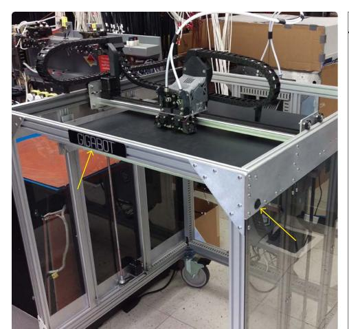
If you are looking at the front of your Gigabot (you should see the Gigabot nameplate) the power switch is located on the right side of your bot closer to the front. It is a small black circle switch; flip it on!
