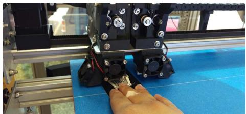
Use the 8mm combination wrench to gradually tighten the M5x12 hex head screws at each corner. Periodically use the business card again to check the level, since tightening the hardware on the rails may have caused them to move slightly. The bed cross rails should be secured and acceptably level to the nozzle after 2-3 total passes.
