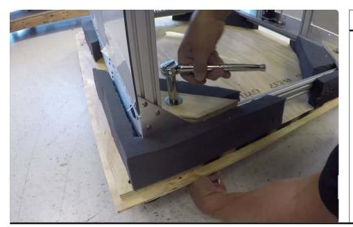
Remove all 4 wooden corner braces by using 2 9/16" wrenches.
