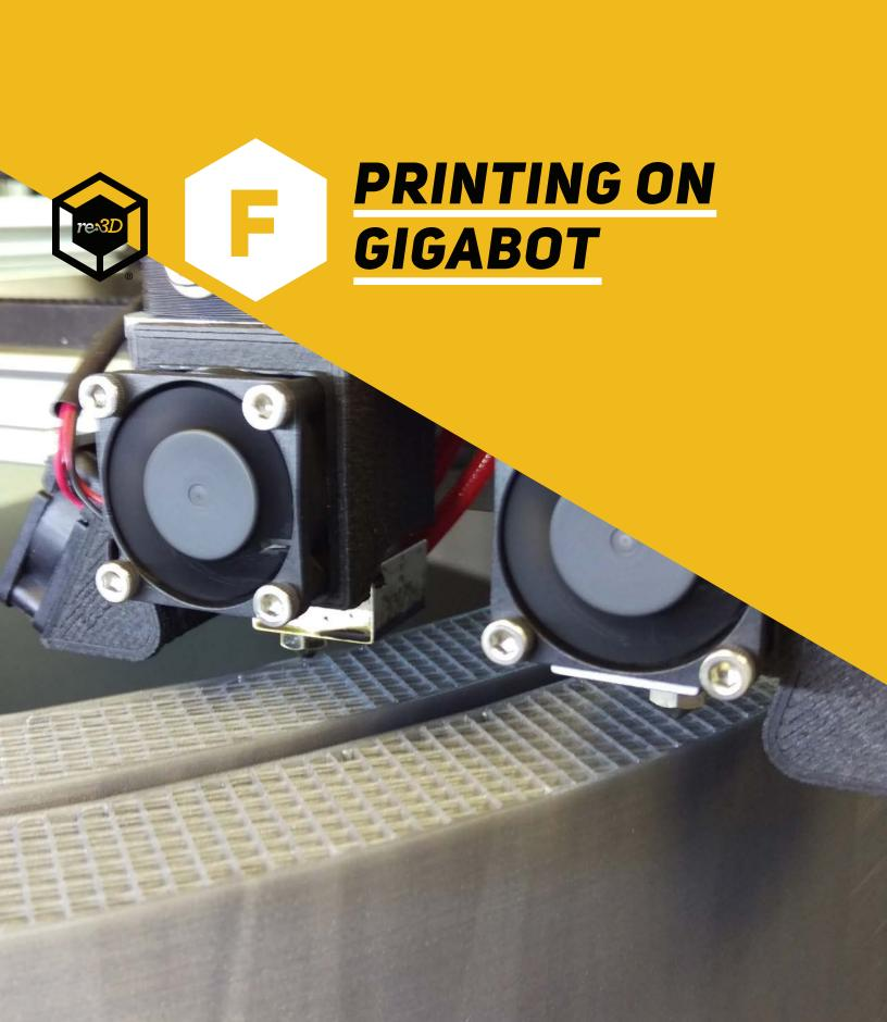
This is it--you're ready to print! There are two ways to make Gigabot® print; via USB or using a microSD card in the Viki LCD controller. Typically, we recommend printing via the microSD card. It's the most reliable method because there is no need to connect to a computer and the USB cable is more susceptible to electrical interference, which can disturb the serial communication to Gigabot®.
