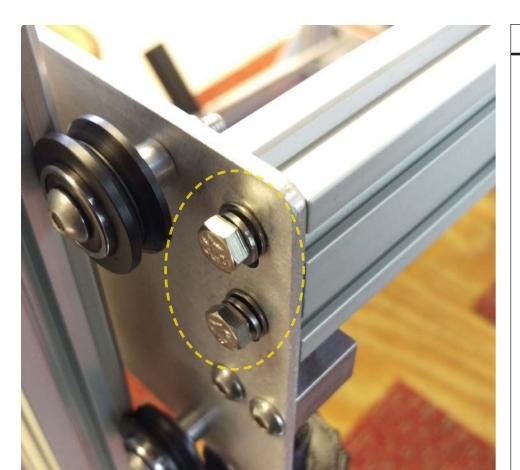
These need to be loose enough so that the ends of the rails can move vertically in the slots of the side plates with little to no resistance.
