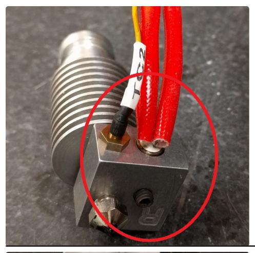
Install M3 threaded thermocouple into hot end -- DO NOT overtighten, or you will break this! Then, install the heater cartridge into the hot end and tighten the set screw -- DO tighten this, so that the cartridge does not fall out.
