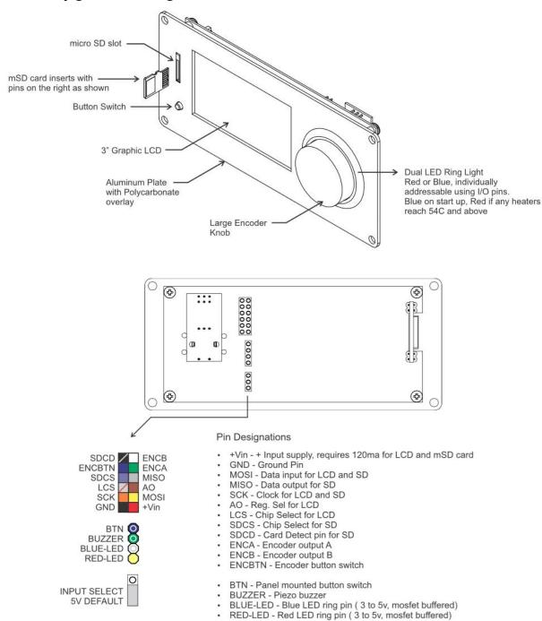
**Note on universal cable** - There are 2 black and 2 gray wires on the cable. To differentiate, one black (SDCD) is marked with a white stripe near the single dupont connector and one gray wire(LCS) is marked with a red stripe. Both are illustrated in this guide as the following color boxes.
