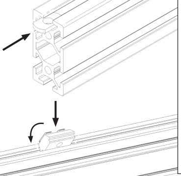
T-nuts are an essential part of assembling the Gigabot®. These are inserted into the aluminum extrusion in order to fasten parts to the frame.
