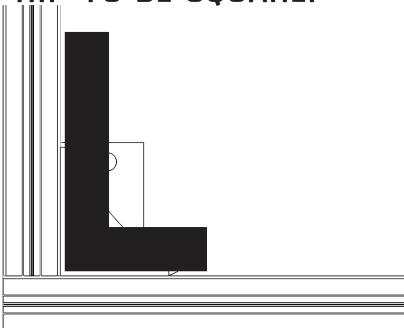
When assembling the Gigabot®, it is essential to work on a flat surface and to carefully square perpendicular parts as much as possible. This is especially important while assembling the side plates, Z-axis uprights and vertical common rails, bed frame, upper and lower cross rails, and bridge assembly. Use large clamps to help square up frames if needed.
