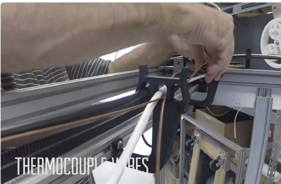
HEAD CABLE (INCLUDES FANS AND HEATER CARTRIDGE WIRES)
