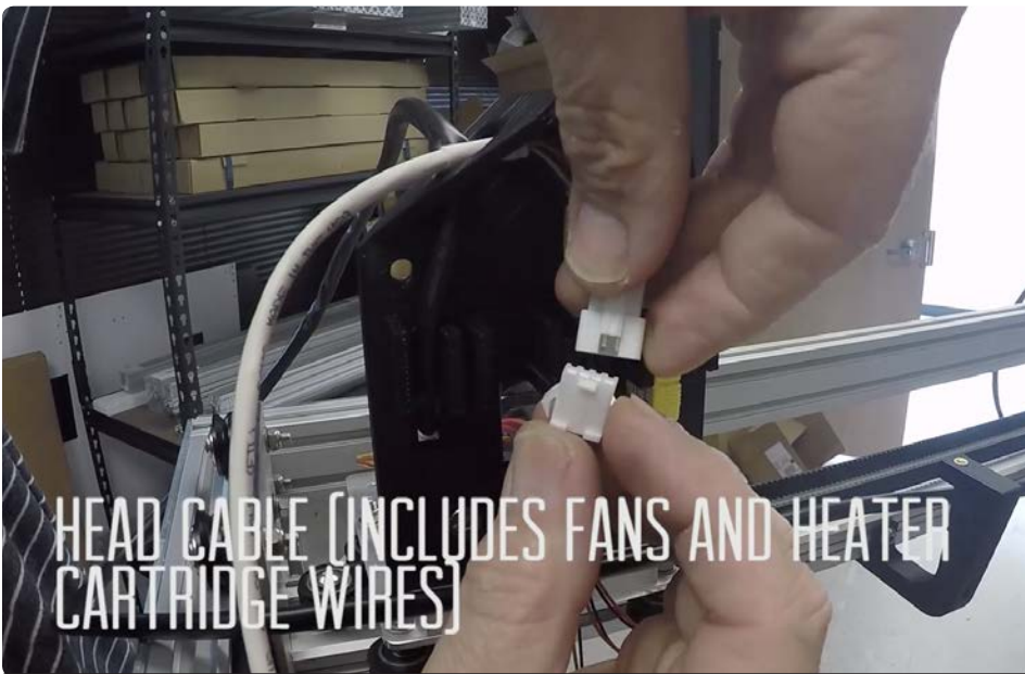
HEAD CABLE (INCLUDES FANS AND HEATER CARTRIDGE WIRES)
