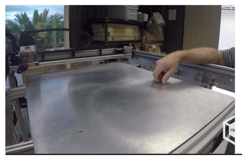
The screw should engage the limit switch before the hot ends can contact the bed. If this is not the case, be prepared to manual engage the upper Z limit switch to avoid damaging your hot end.
